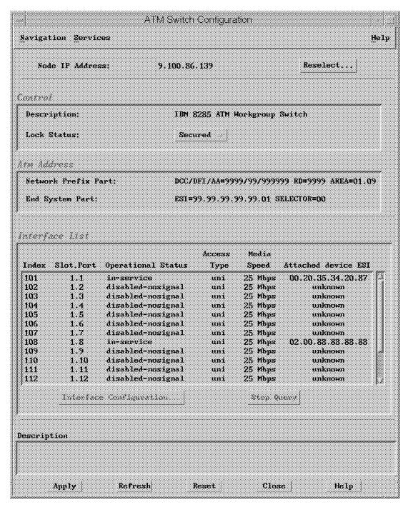
Figure 53. IBM 8285 Node Configuration Panel
